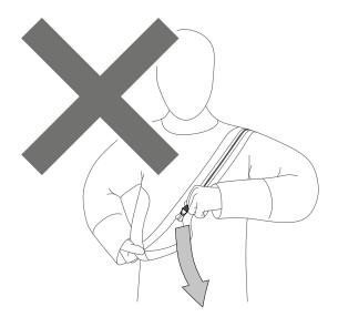
**DO NOT** pull the zipper away from your body. **DO NOT** pull the zipper at an oblique angle to the zip run **DO NOT** use excessive force.
