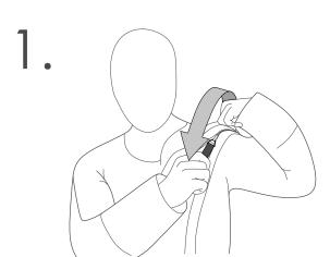
Brace the top of the drysuit directly above the AQUASEAL® Zip. Take hold of the zipper toggle and pull downwards following the line/run of the zip.
